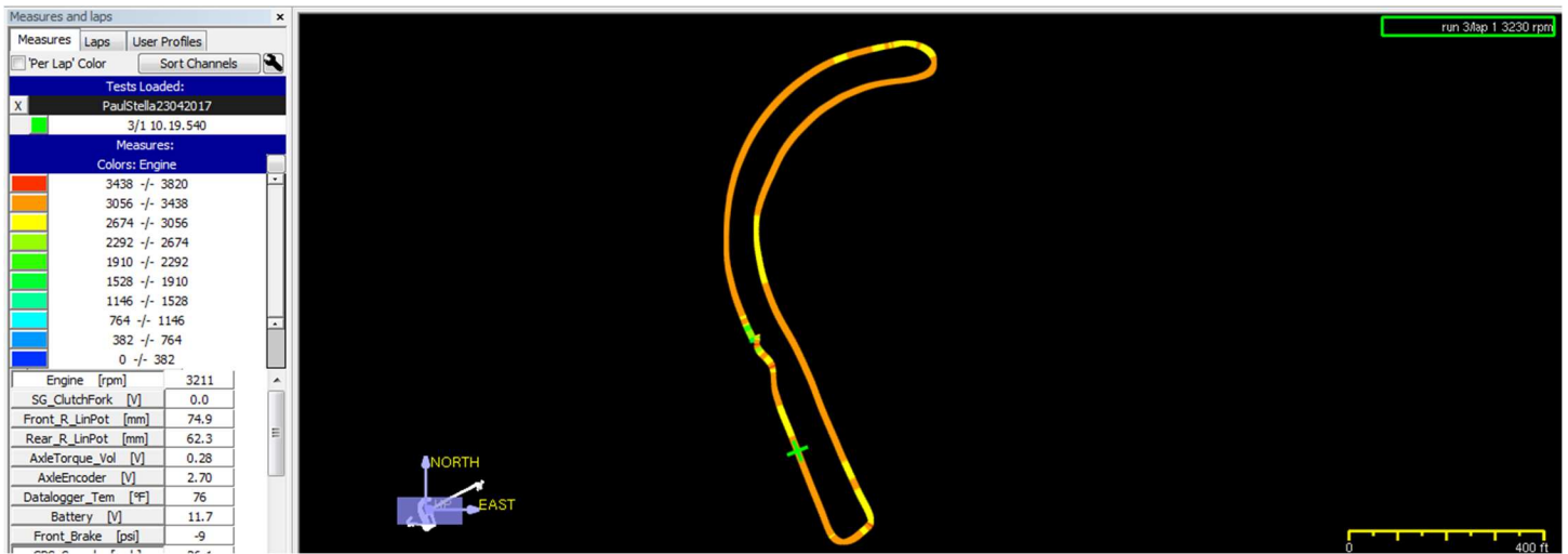
Figure 68: J-Lot acceleration and cornering GPS data displaying engine RPM
