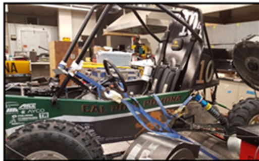
Figure 61: 2017 Baja car strapped to chassis dyno
