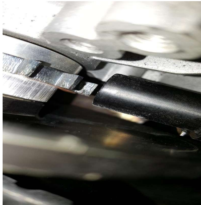
Figure 20: Implementation of Hall Effect and tone ring for the prototype CVT
